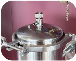
Screw the valve onto the housing cover.
