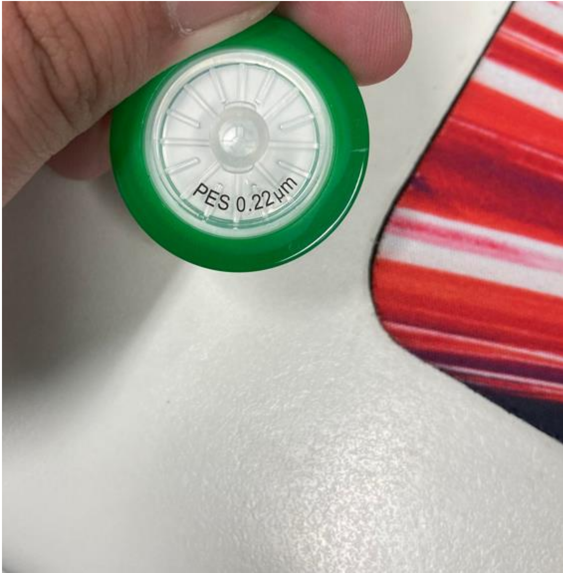
Appendix Figure A 3: Photo of syringe filter used to process water samples for the IC
