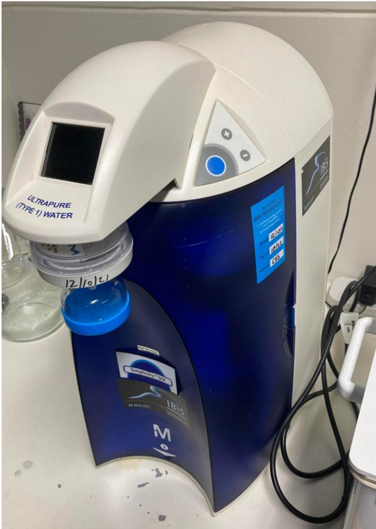
Appendix Figure A 4: Photo of filter used to obtain Type 1 Ultrapure water
