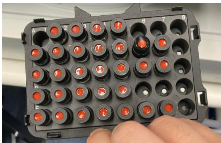
Figure 2: A picture of an IC's autosampler tray with samples inserted
