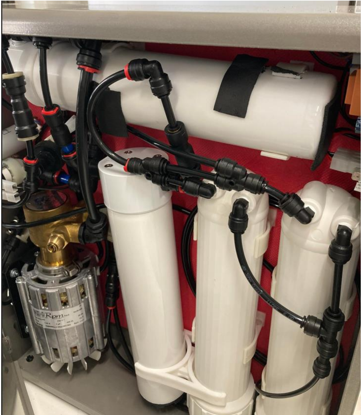
Appendix Figure A 6: Photo of the interior of EVOFILTER. The top tube contains the RO membrane and the 3 columns at the bottom right house the pre-treatment modules
